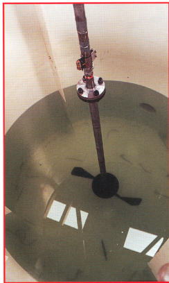
Laboratory strain gauge analysis on new impeller
